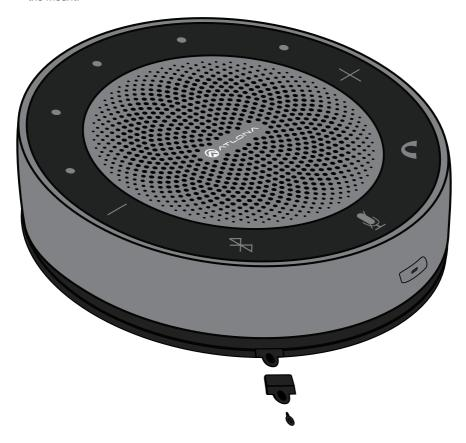
Attach the previously removed detachable lip with the screw from the first step. This will secure the unit to the mount.
