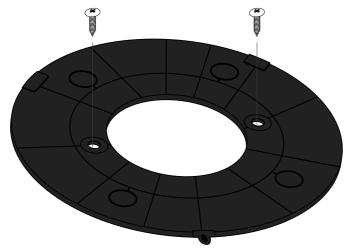
b. Remove the paper from the top of the included adhesive ring (included with AT-CAP-SP100-MNT) and press it firmly to the bottom of the mount. Once done, remove the paper from the bottom of the adhesive ring and press the secure mount (adhesive side down) onto the table/surface for 15 seconds to ensure the mount is secure.
